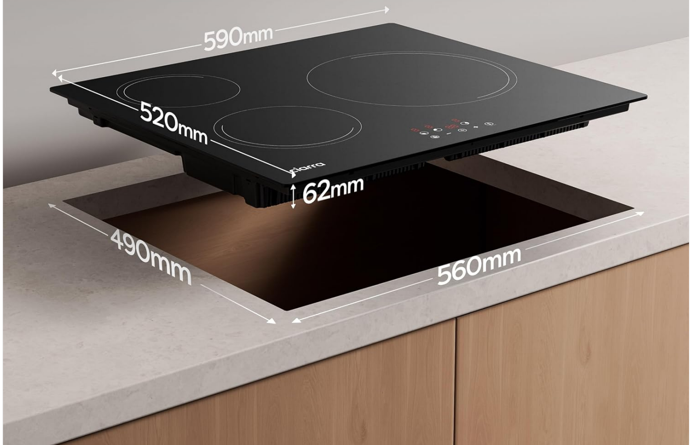
Image 4.1: Diagram showing the CIARRA CABBIH3-E Induction Hob being installed into a countertop, with precise measurements for the hob (590mm x 520mm x 62mm depth) and the required cut-out (560mm x 490mm).
