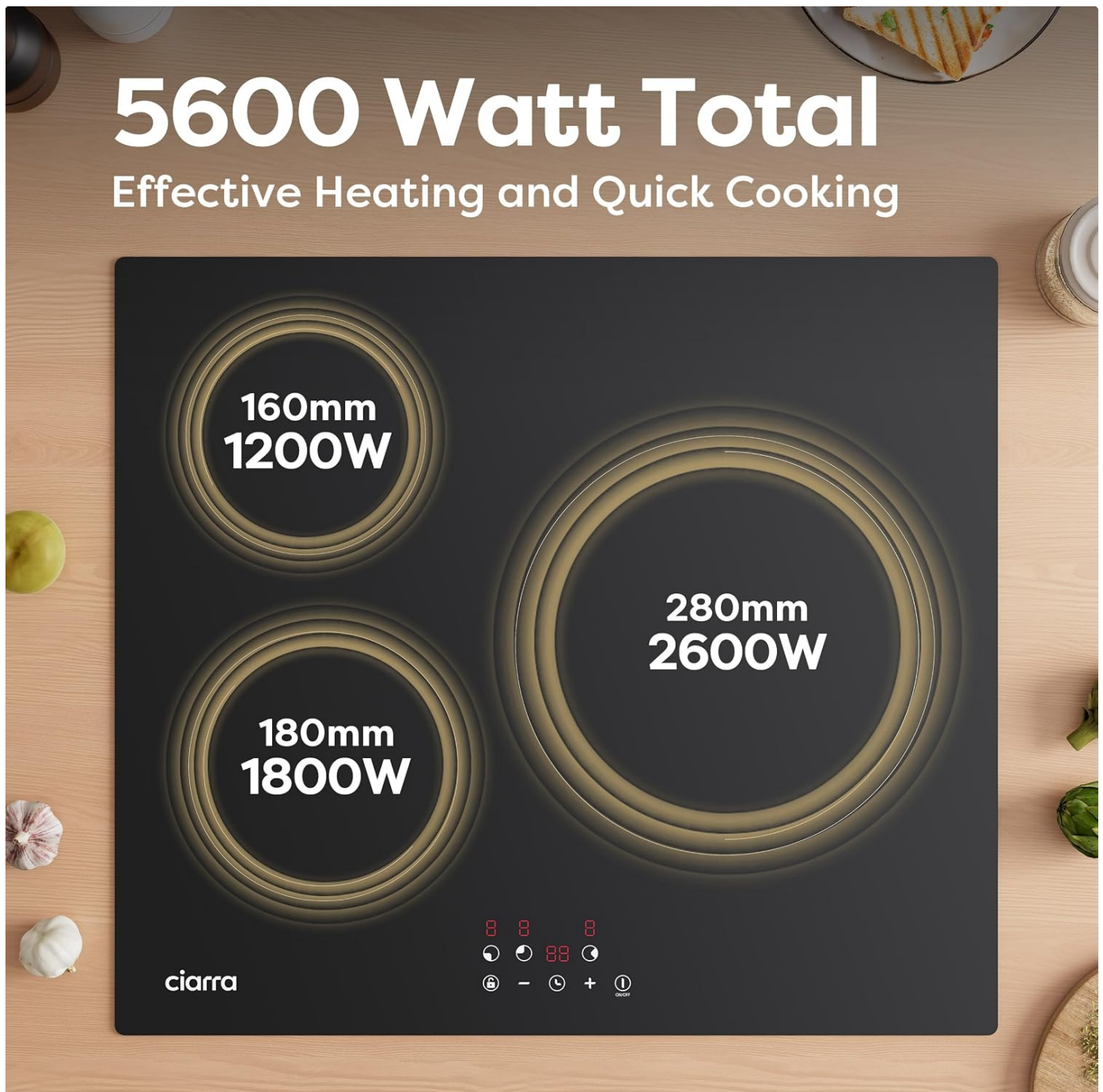
Image 3.1: Diagram illustrating the three cooking zones of the CIARRA CABBIH3-E Induction Hob, detailing their diameters (160mm, 180mm, 280mm) and corresponding wattage (1200W, 1800W, 2600W).
