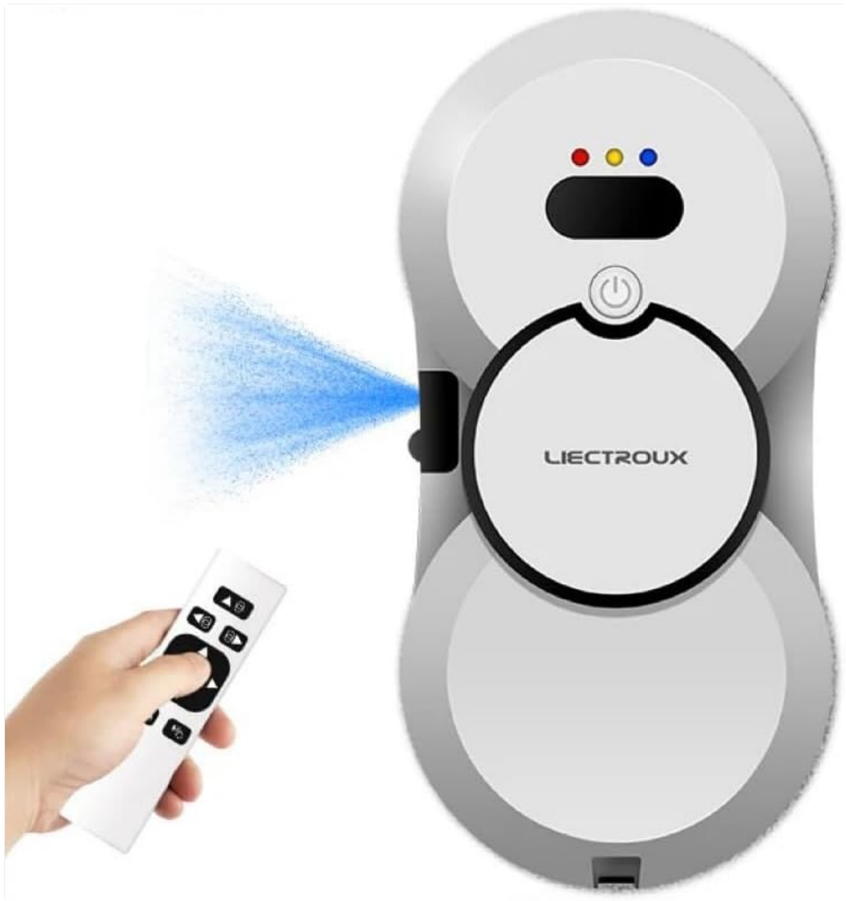
Figure 3: The LIECTROUX HCR-10 robot and its remote control, illustrating the ultrasonic water spray function.
