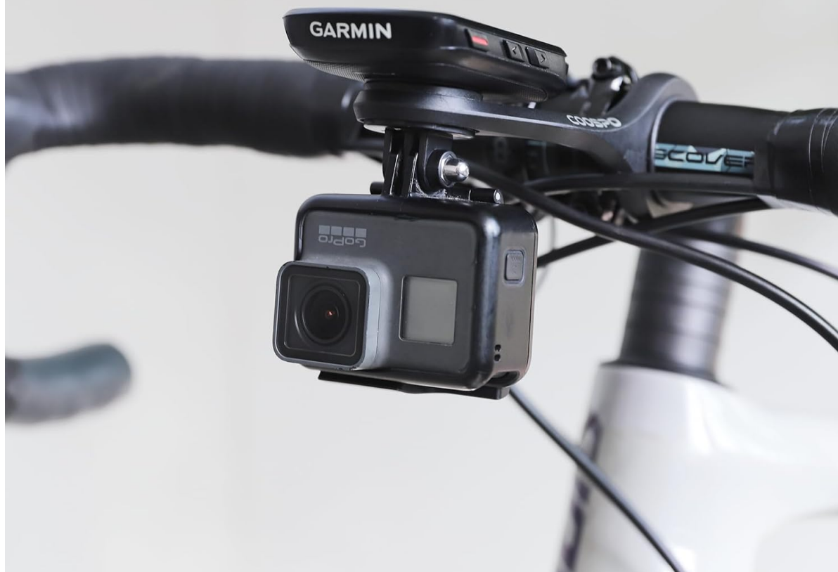
Image 6.1: The mount in operation, holding both a bike computer and an action camera.
