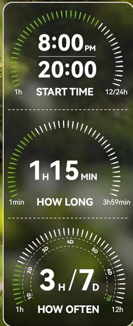
Figure 6: Visual representation of the three timed watering cycle modes: start time, duration, and frequency options.
