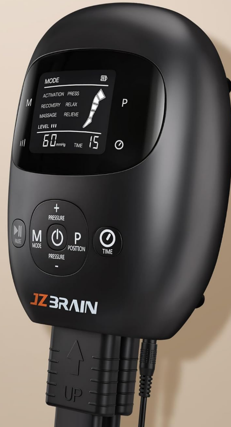
Image: Detailed view of the Smart Digital Controller for mode, intensity, and timer selection.
