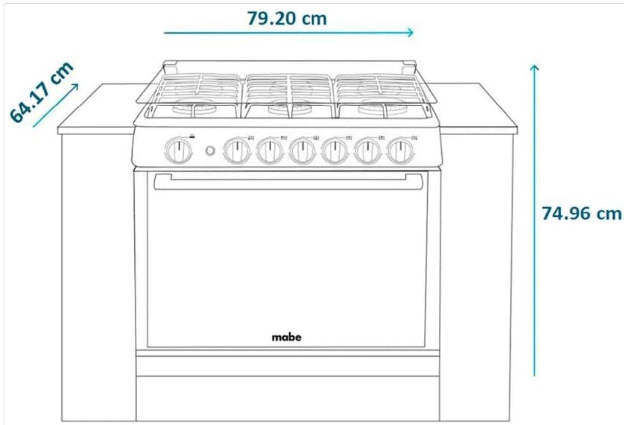
**Image Description:** A technical diagram illustrating the front view of the Mabe MA0C80400CI0 built-in stove with key dimensions labeled. The width is approximately 79.20 cm, the height from the base to the cooktop is 64.17 cm, and the total height including the back panel is 74.96 cm. This diagram is essential for proper cabinet cutout and installation planning.
