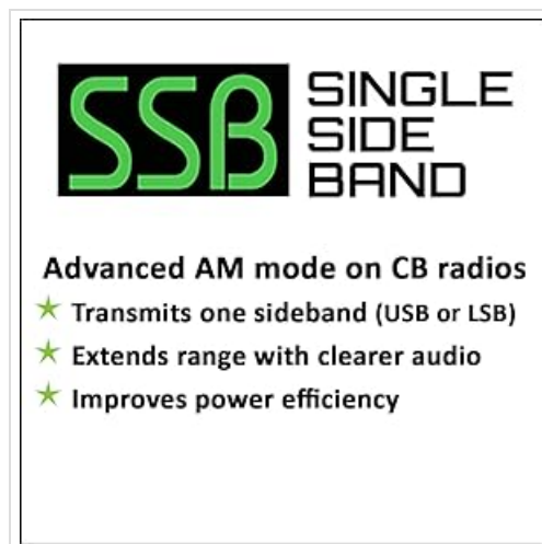
Figure 4: Explanation of Single Side Band (SSB) mode.
