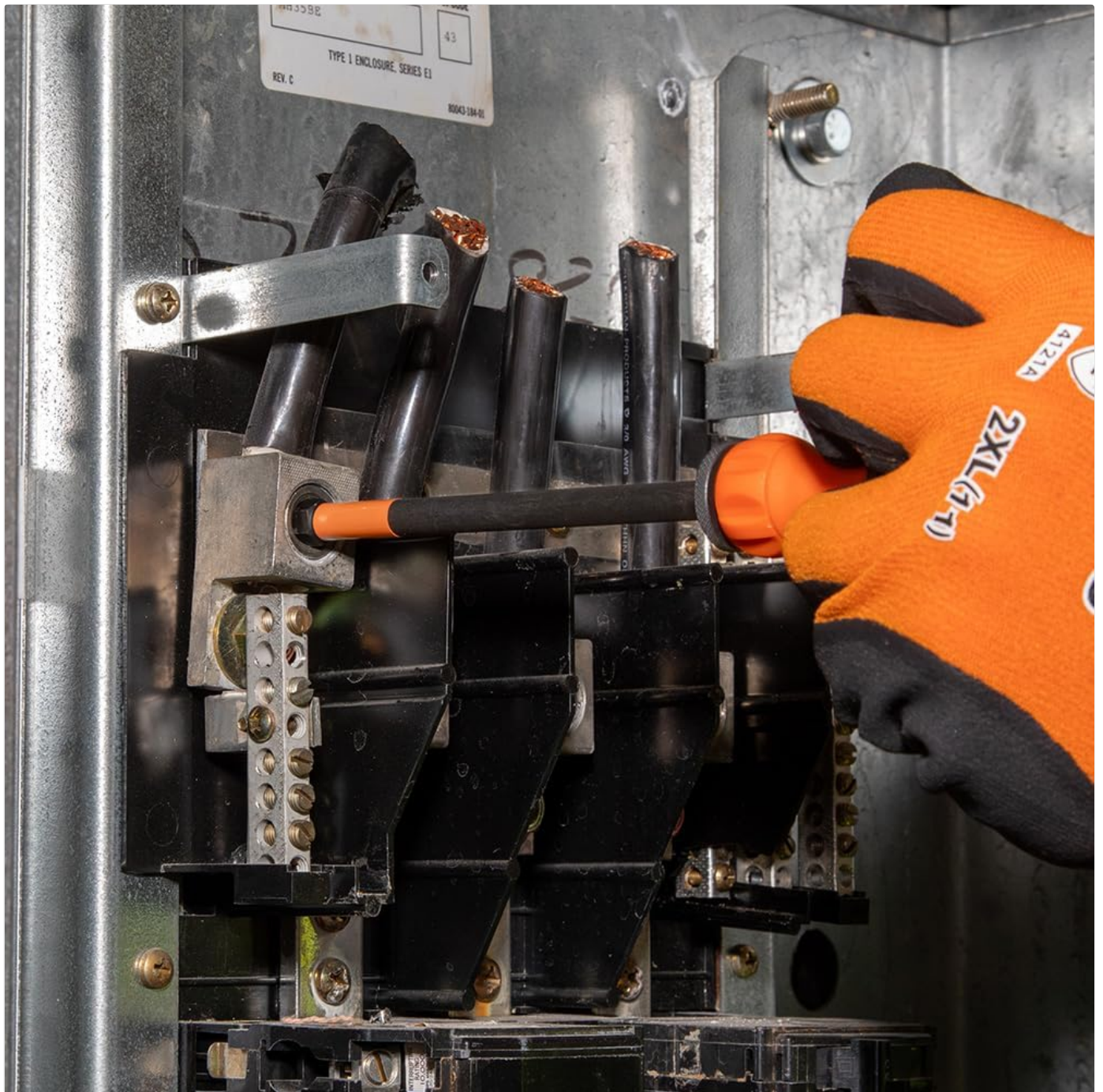
Using an extended bit for reaching fasteners in deep spaces.
