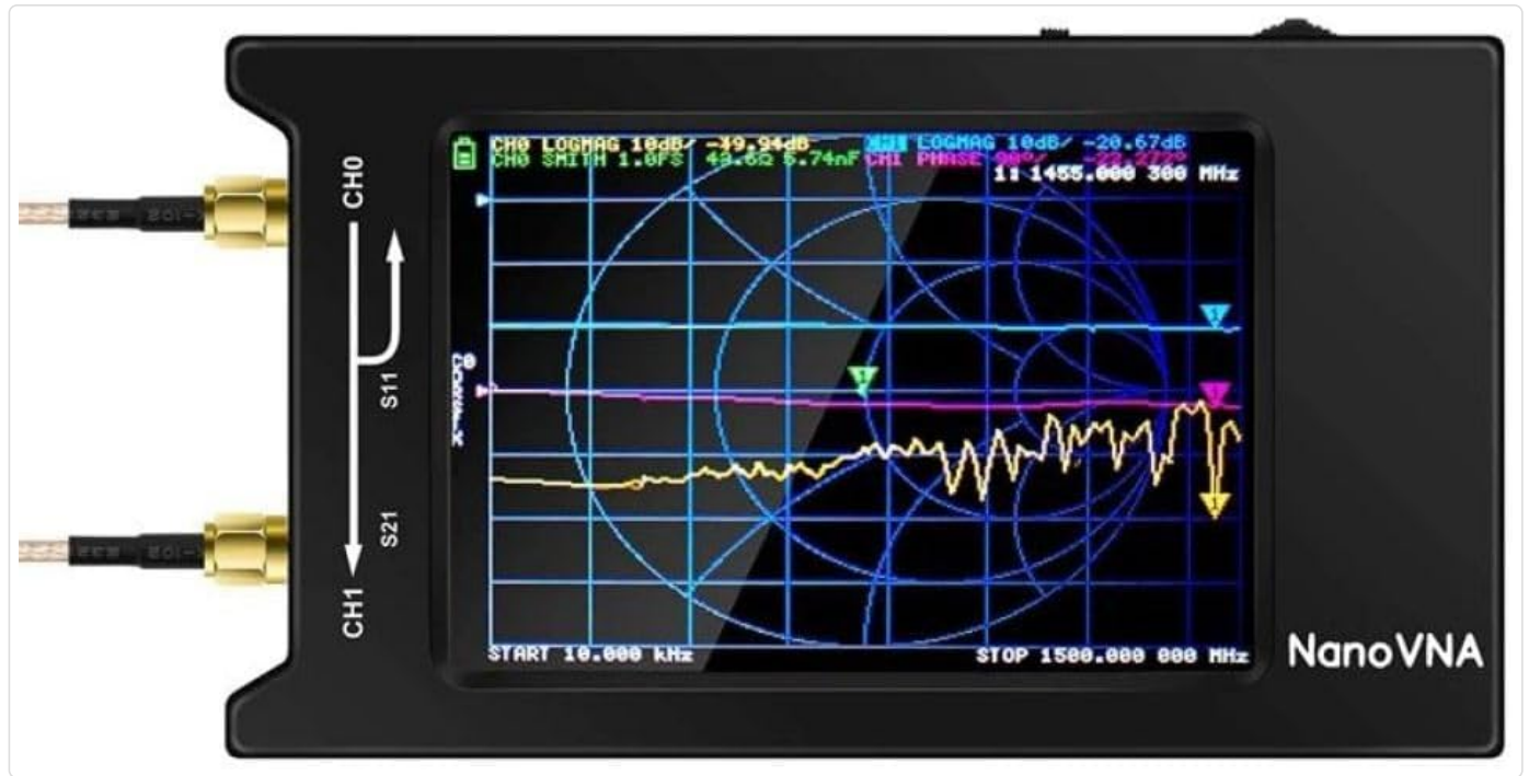
Figure 4.2.1: NanoVNA-H4 device showing CH0 and CH1 ports for RF connections.
