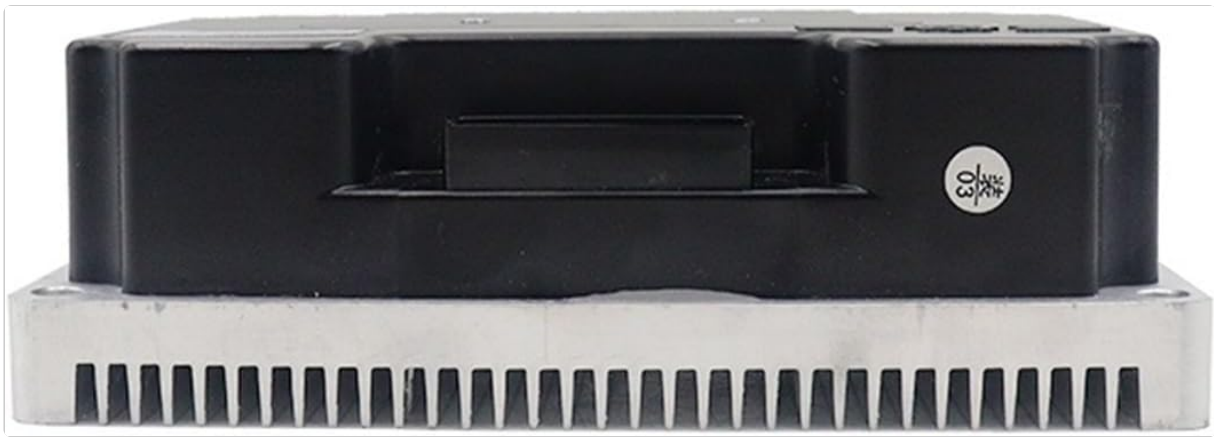
Figure 5: Side view of the SHHJCO Far-Driver V2 Controller ND72340, highlighting the heat sink fins for thermal management.
