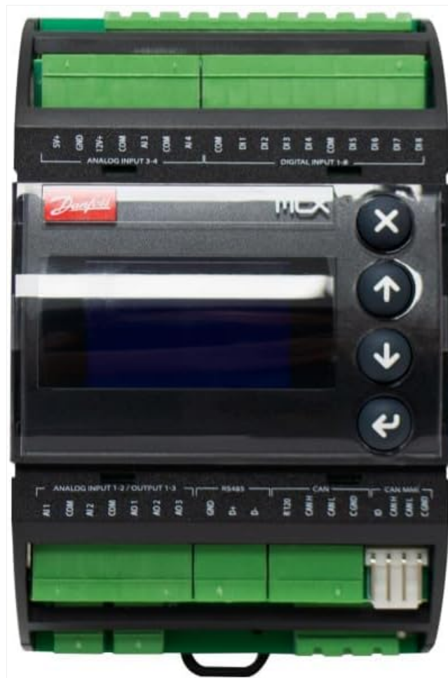
Figure 2.2.1: Front view of the Danfoss MCX06D Programmable Controller. This image displays the main unit with its central display screen, four control buttons (X, Up, Down, Back), and clearly labeled green terminal blocks for analog inputs, digital inputs, and communication ports (RS485, CAN).
