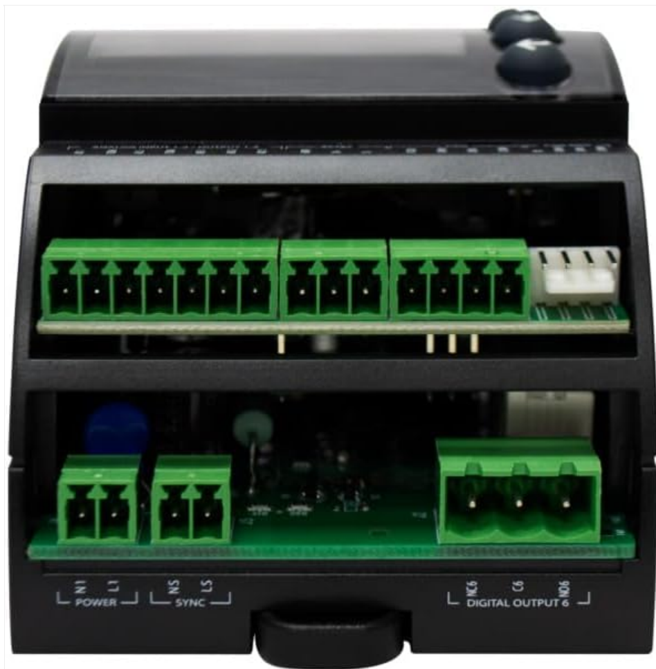
Figure 2.2.2: Top-down view of the Danfoss MCX06D Programmable Controller. This image highlights the upper section of the controller, detailing the green terminal blocks for analog inputs (S+, GND, AI1, AI2, AI3, AI4) and digital inputs (DI1 through DI8), along with their common (COM) connections.
