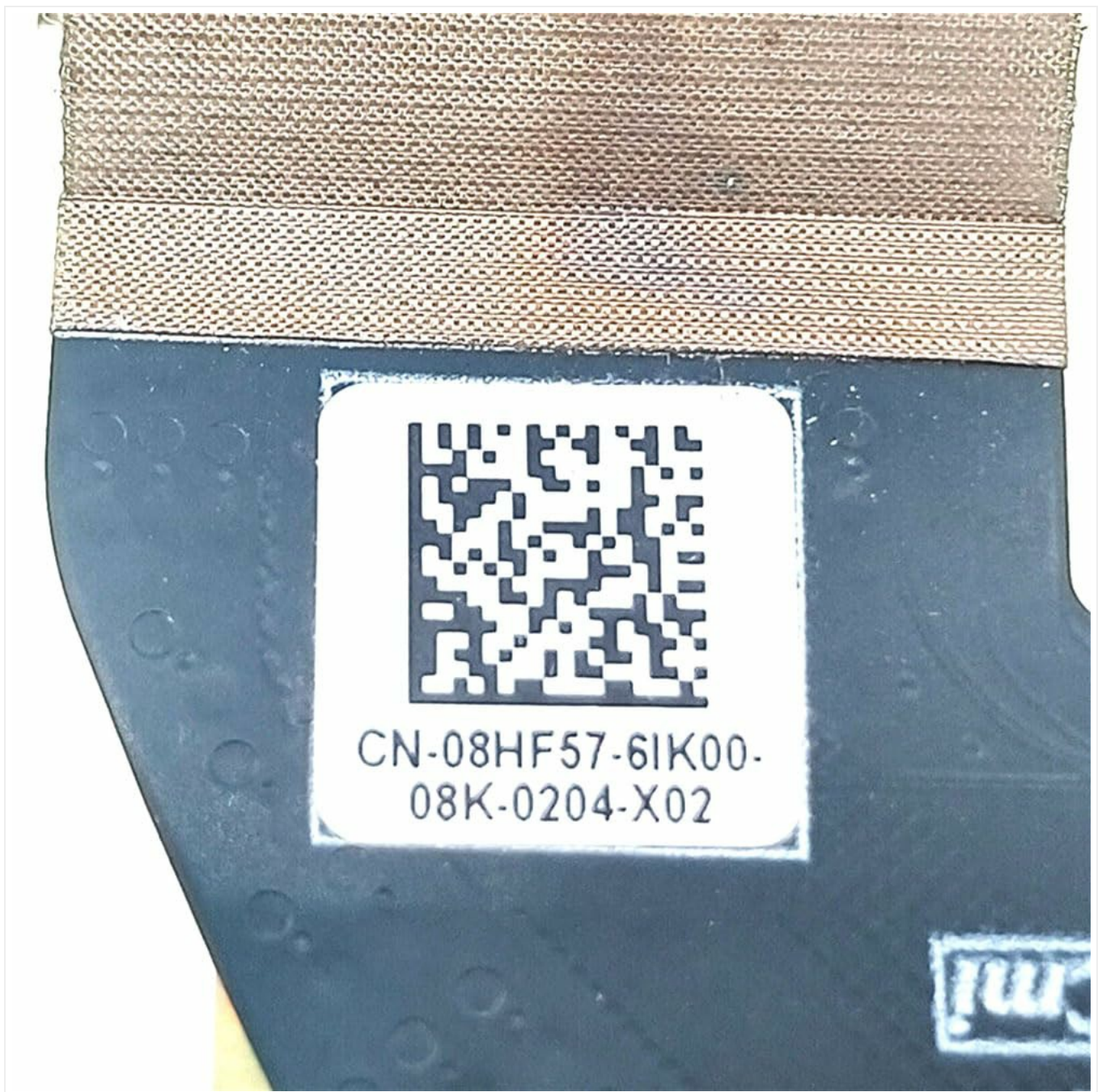
Figure 3.3: Close-up view of the cable's identification label, showing the part number (CN-08HF57-6IK00-08K-0204-X02) and a QR code. Verify these numbers against your original cable or laptop's service manual to ensure compatibility.
