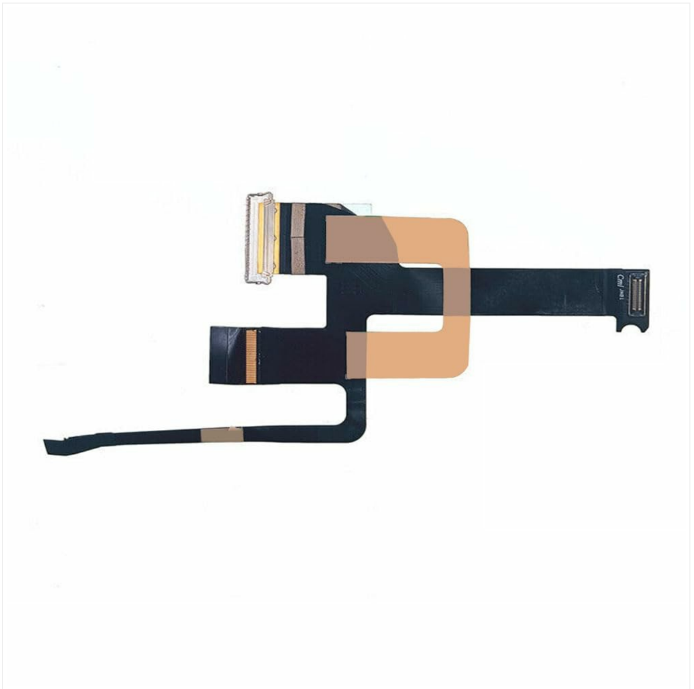
Figure 3.2: Another perspective of the LVDS cable, highlighting the different sections and the delicate nature of the connectors. This view helps in understanding the cable's routing within the laptop chassis.
