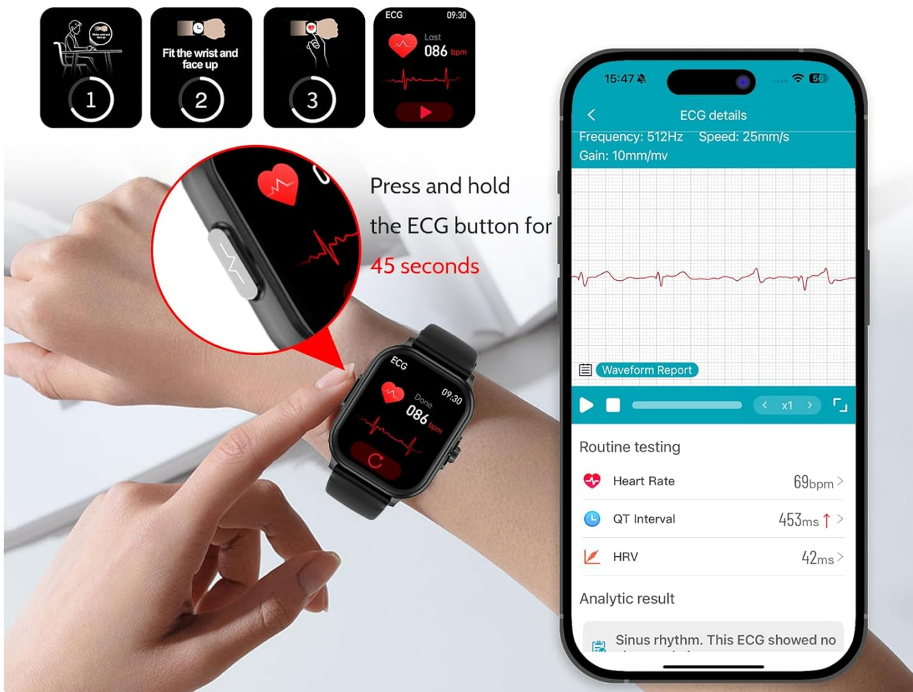
Image: A visual guide on how to perform an ECG measurement using the smartwatch and view the report in the app.
