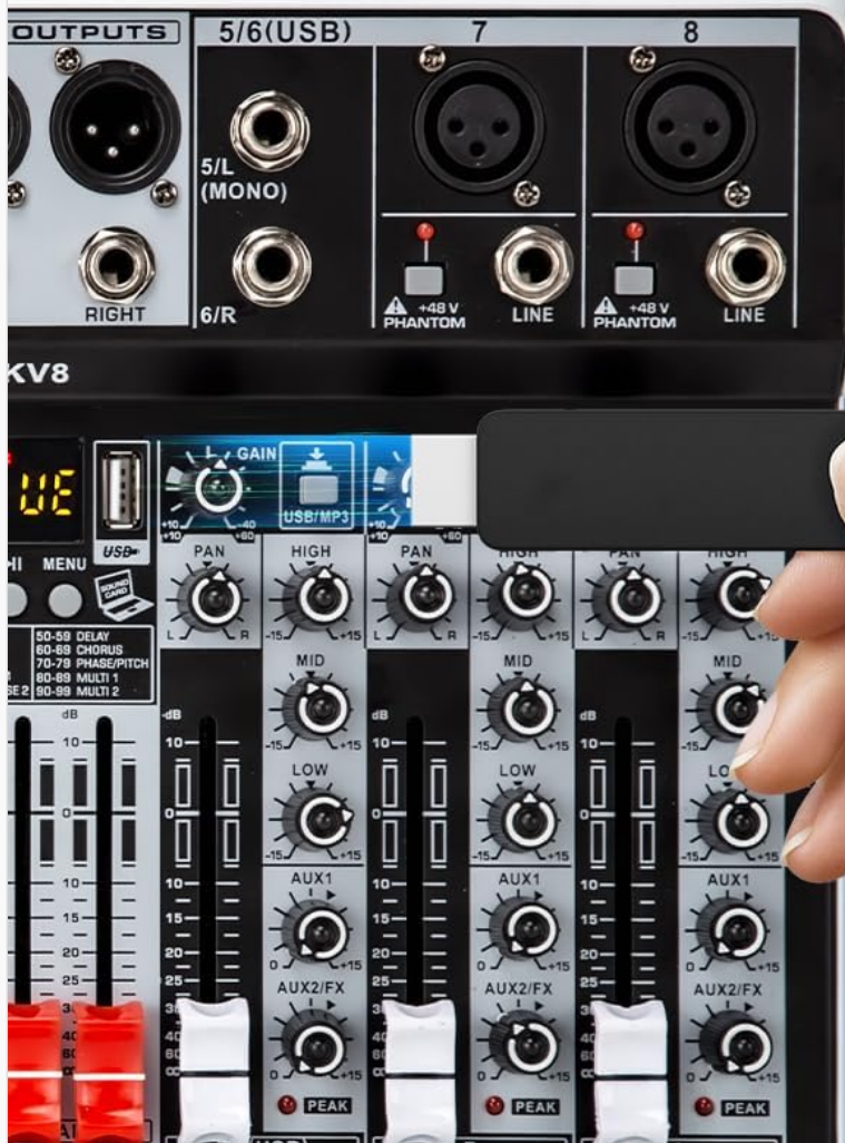
Figure 2: +48V Phantom Power Activation
