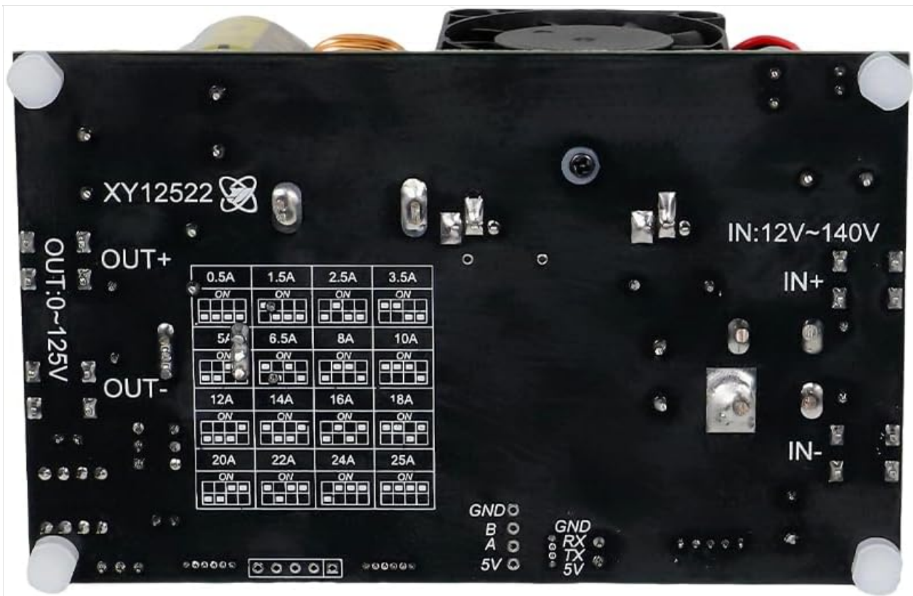
Figure 3: Bottom view of the module with input/output terminals and DIP switches.
