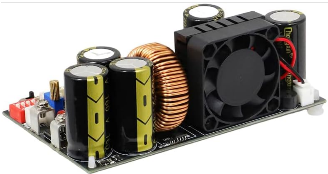
Figure 2: Angled view of the DC Buck Converter, highlighting the cooling fan.
