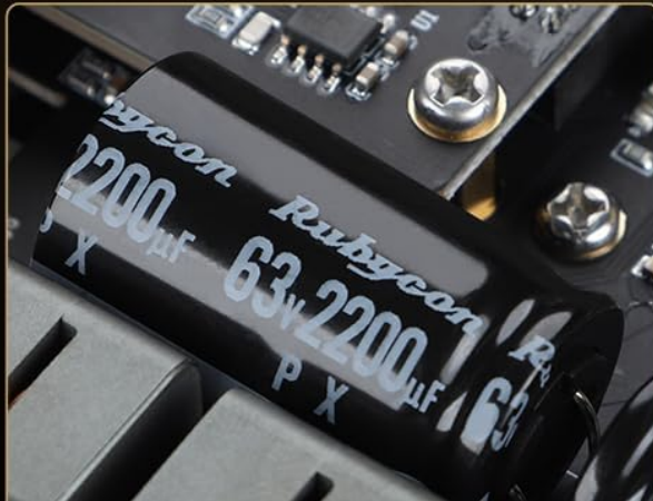
Rubycon 63V2200uf filter capacitor
