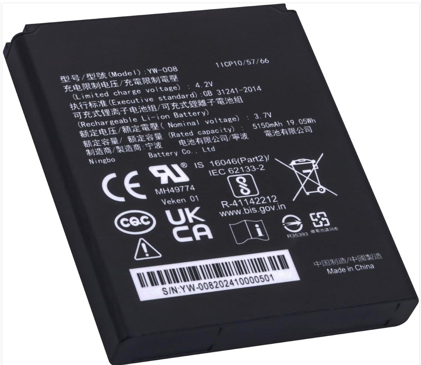
Image 1.1: The DFTIM YW-008 Li-ion Battery. This image displays the front side of the black rectangular battery, showing its model number, voltage, capacity, and various certification marks.
