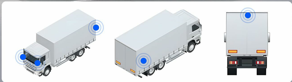
Image: Diagram illustrating optimal placement of the five cameras on a large vehicle for 360-degree full view coverage, including front, rear, and side perspectives.
