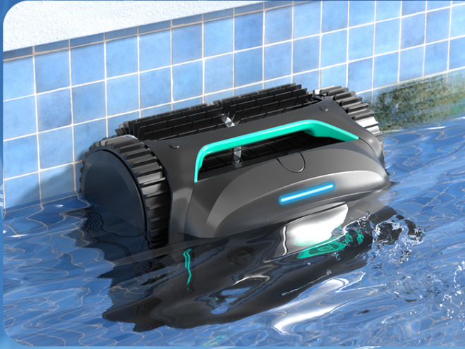
Figure 4.3: The WYBOT C2 demonstrating its wall cleaning function underwater.
