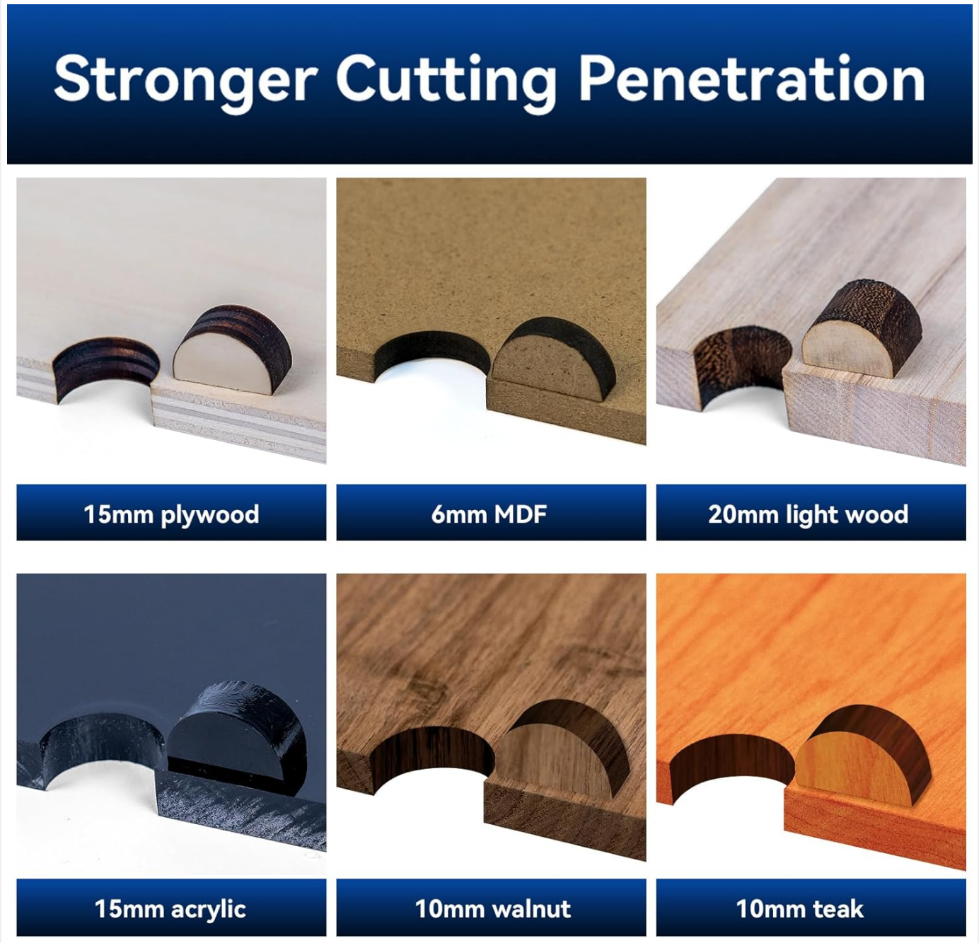
Figure 7: Examples of cutting depth on various materials like plywood, MDF, light wood, acrylic, walnut, and teak.
