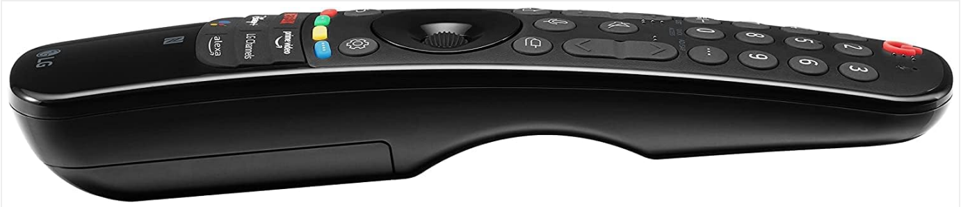
Figure 4.1: Side view of the AN-MR22GA Magic Remote Control, illustrating the location of the battery compartment.
