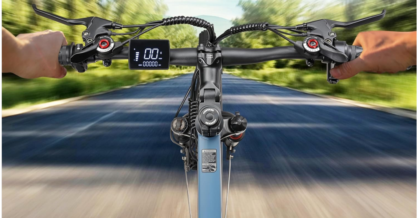
Figure 5: The LCD display provides clear information including current speed, battery level, riding mode, and distance traveled. It also offers lighting control and allows selection between the 3 riding modes.
