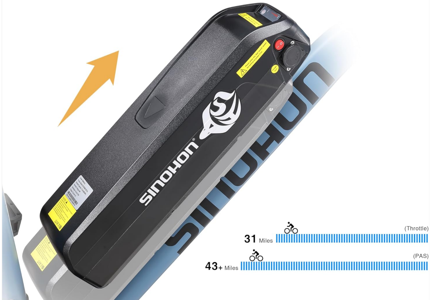
Figure 2: The 48V 12.5Ah (600Wh) removable lithium battery offers a range of 40+ miles. It includes UL certification for security and a Battery Management System (BMS) for intelligent safety. Charging time is approximately 6-8 hours with the included 3A fast charger.
