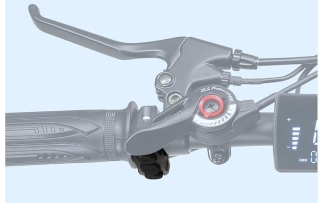
Figure 4: The EM200 offers four distinct riding modes: Twist Throttle for pure electric power, Pedal-Assisted for a boost while pedaling, Just Pedaling for traditional cycling, and a Power Assist Walking Mode for easier maneuvering when walking alongside the bike.
