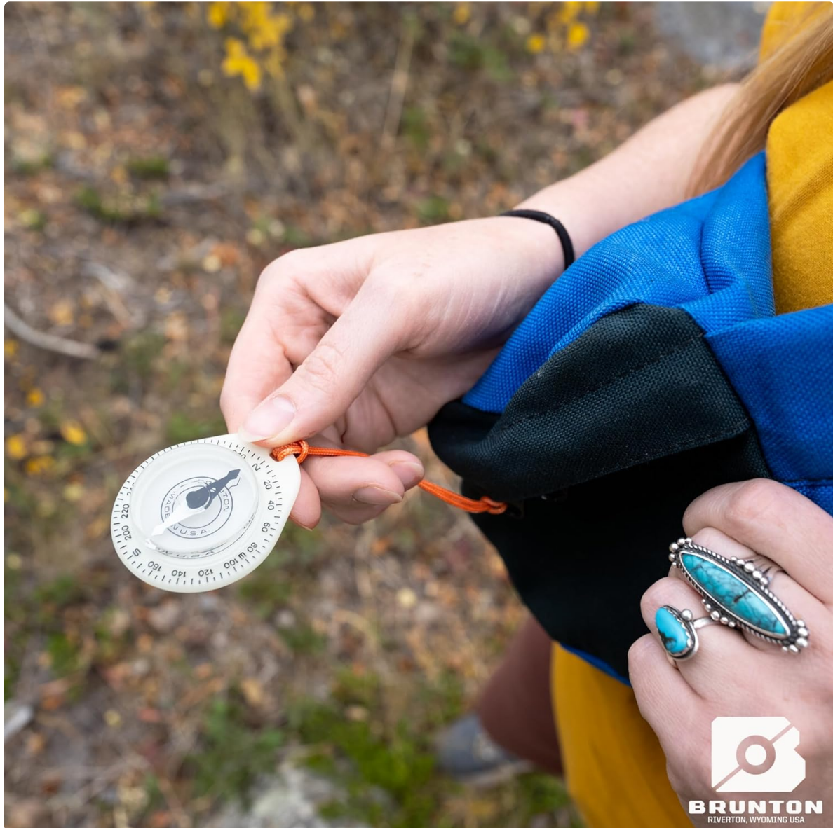
Figure 4.1: Proper way to hold the compass for accurate readings.
