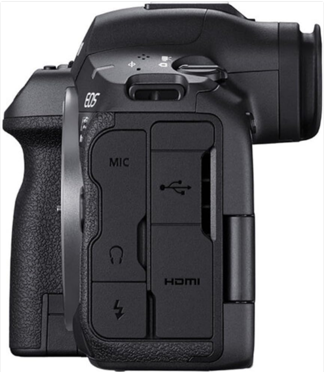
Image 4: Side Ports. This image details the various connectivity ports on the side of the camera, including microphone input, USB-C, and HDMI output.
