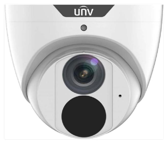
This image displays the front view of the UNV UN-IPC3618SB-ADF28KM-I0 4K 8MP Turret IP Camera, highlighting its lens, IR illuminator, and microphone.
