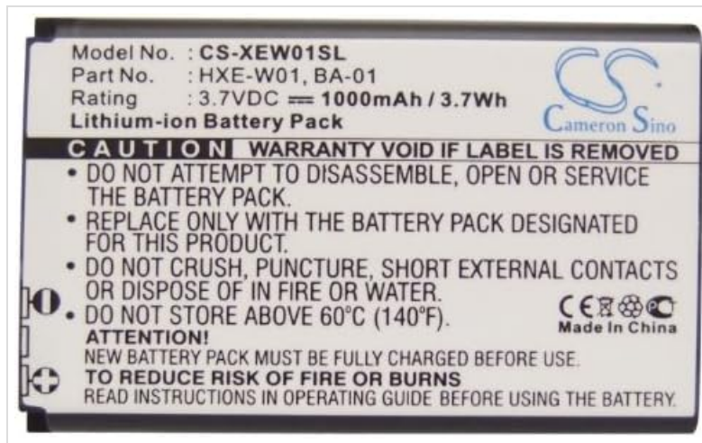
Close-up view of the DCH battery label, showing model number, part number, rating, and critical safety warnings regarding handling and storage.
