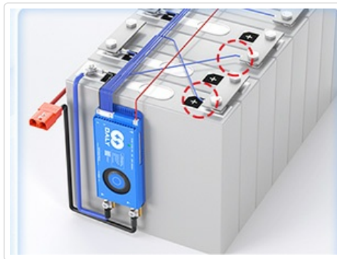
Image 2.3: Cell voltage sensing wire connection.
