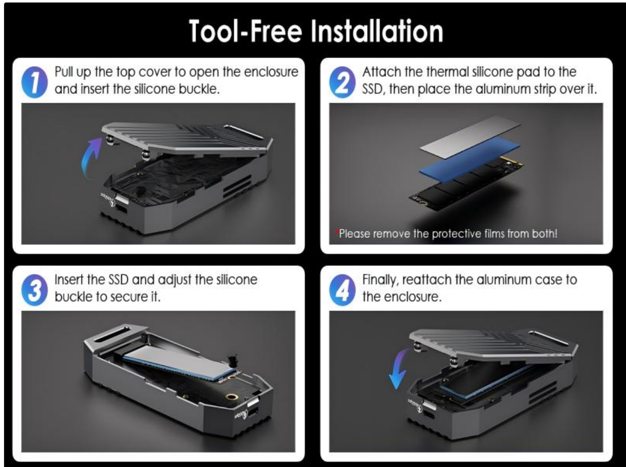
Figure 3: Visual guide for the tool-free installation process of an NVMe SSD into the enclosure.
