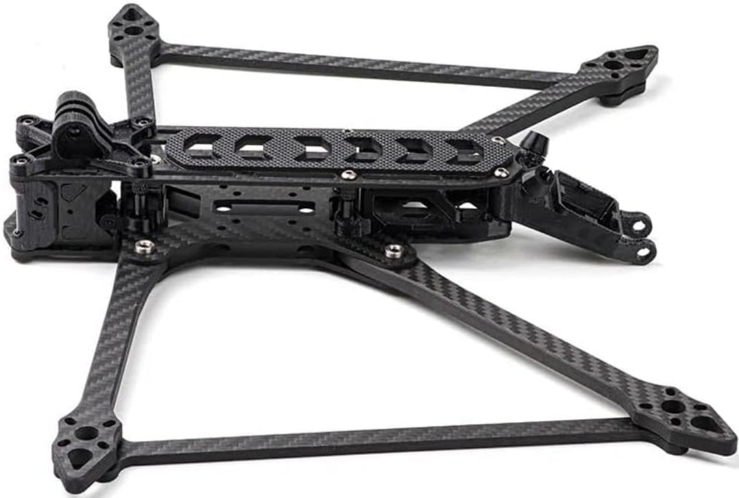
Figure 3: Side view of the frame, showing the layered plate design and mounting points for electronics.
