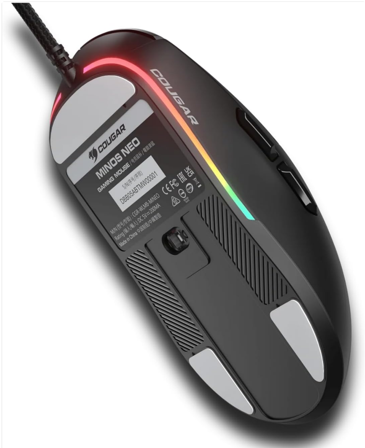
Figure 3.3: Bottom view of the COUGAR Minos Neo RGB Wired Gaming Mouse, displaying the optical sensor, glide feet, and product information label.
