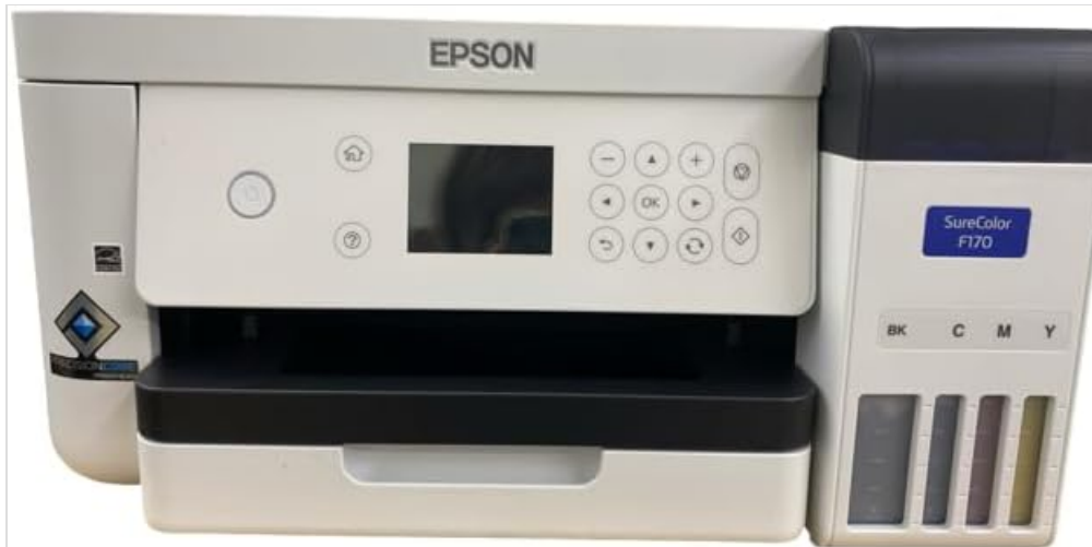
Figure 4.3: Detailed view of the Epson SureColor F170 control panel, showing the LCD screen, power button, navigation buttons, and function keys for printer operation.
