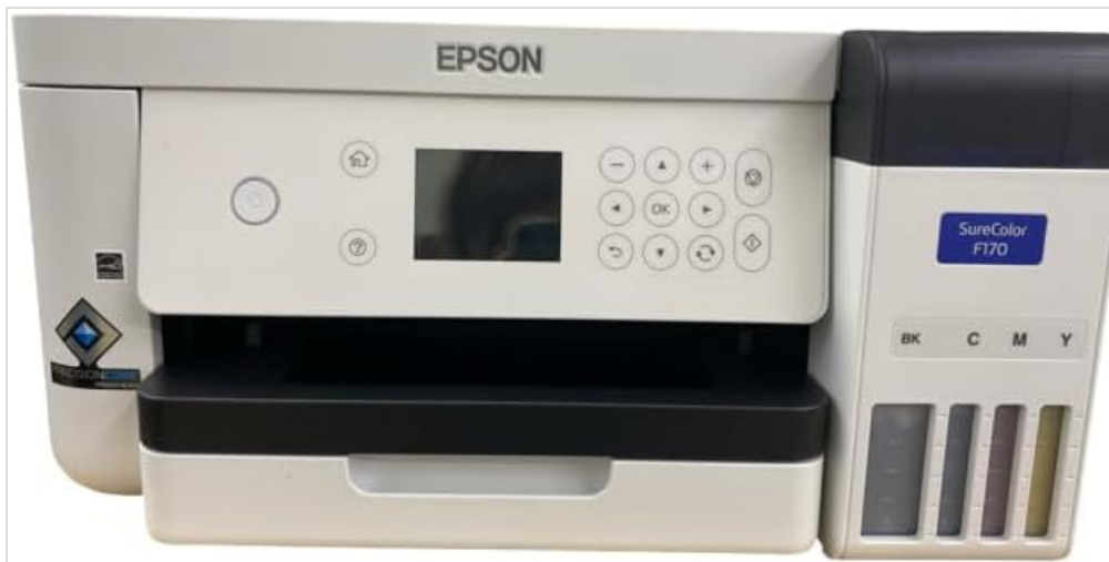
Figure 3.2: Close-up view of the printer's control panel and visible ink tanks, indicating where ink is filled.
