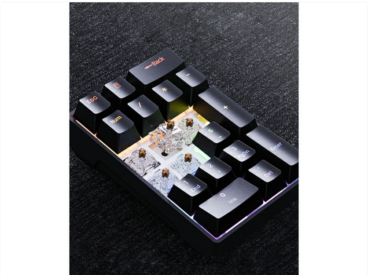
Image 3.2: Mechanical Brown Switches visible under keycaps.
