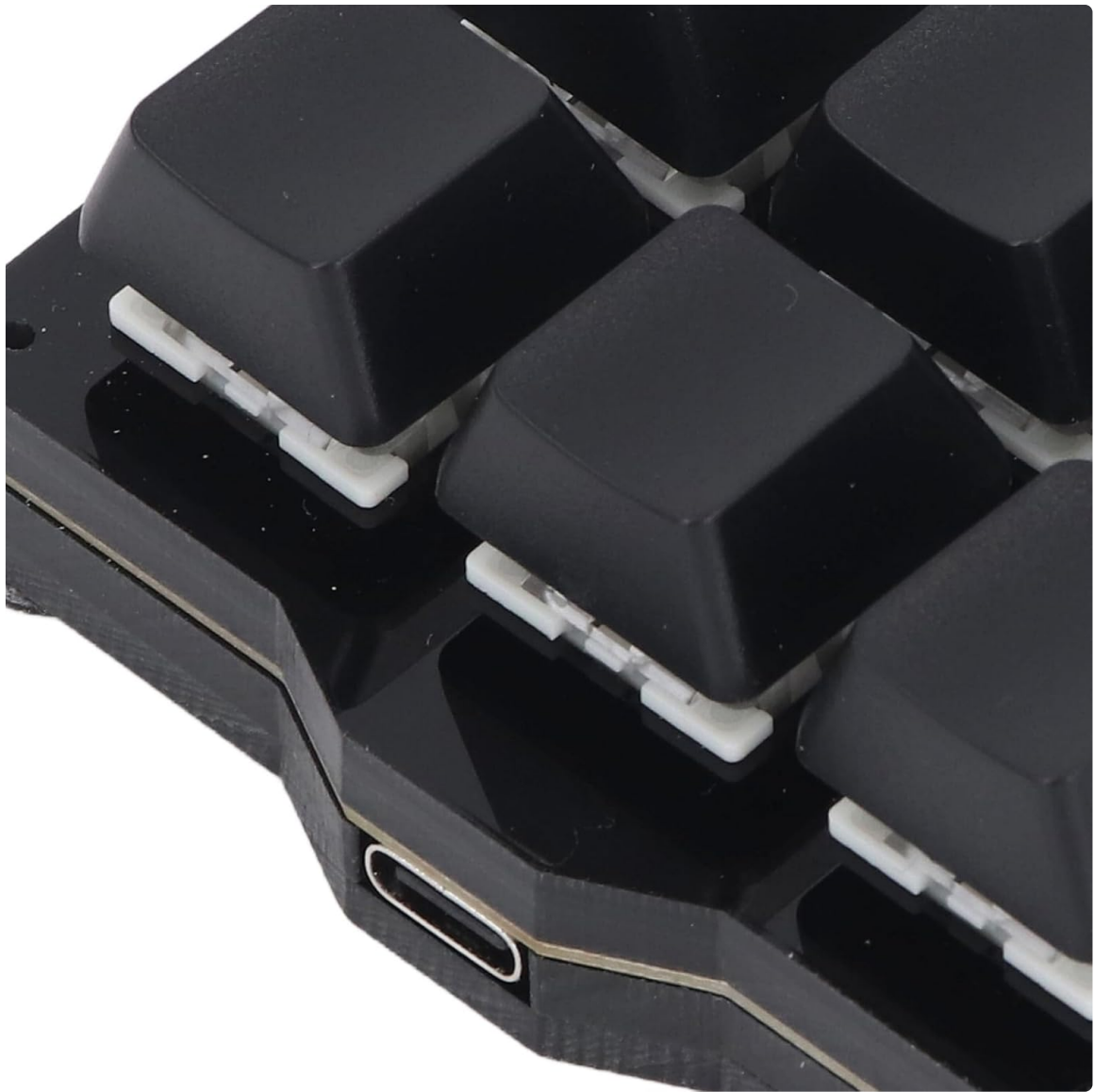
Image: A close-up view of the USB Type-C port located on the side of the keyboard for connection.
