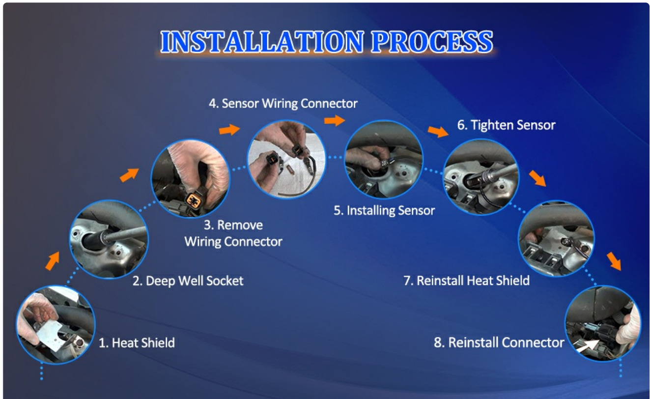
Figure 4.1: Installation Process Overview
