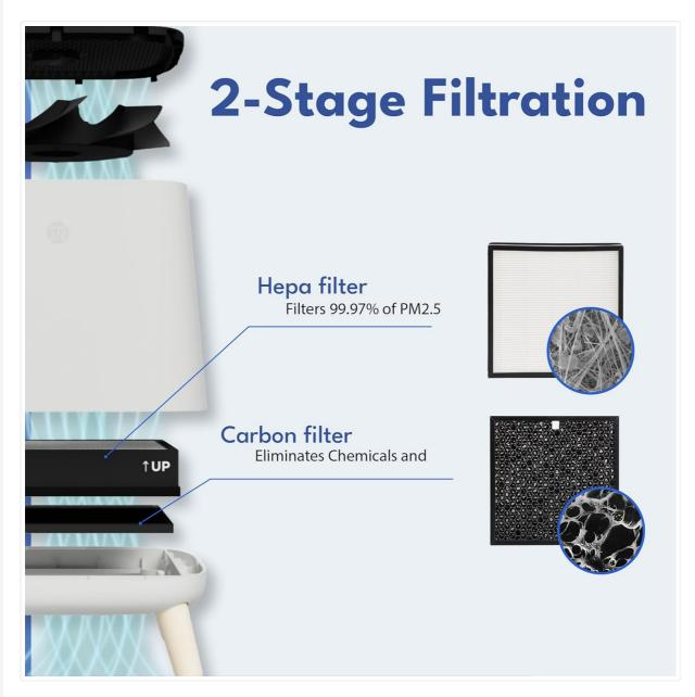
Description: A diagram illustrating the internal components of the Smart Air Sqair air purifier, showing the sequential placement of the HEPA filter and a carbon filter, and how air flows through them for effective two-stage filtration.
