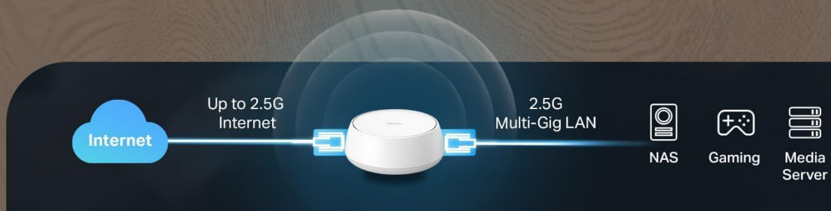
Image: Illustration of a Deco unit connecting to the internet and providing multi-gigabit connectivity to various devices.
