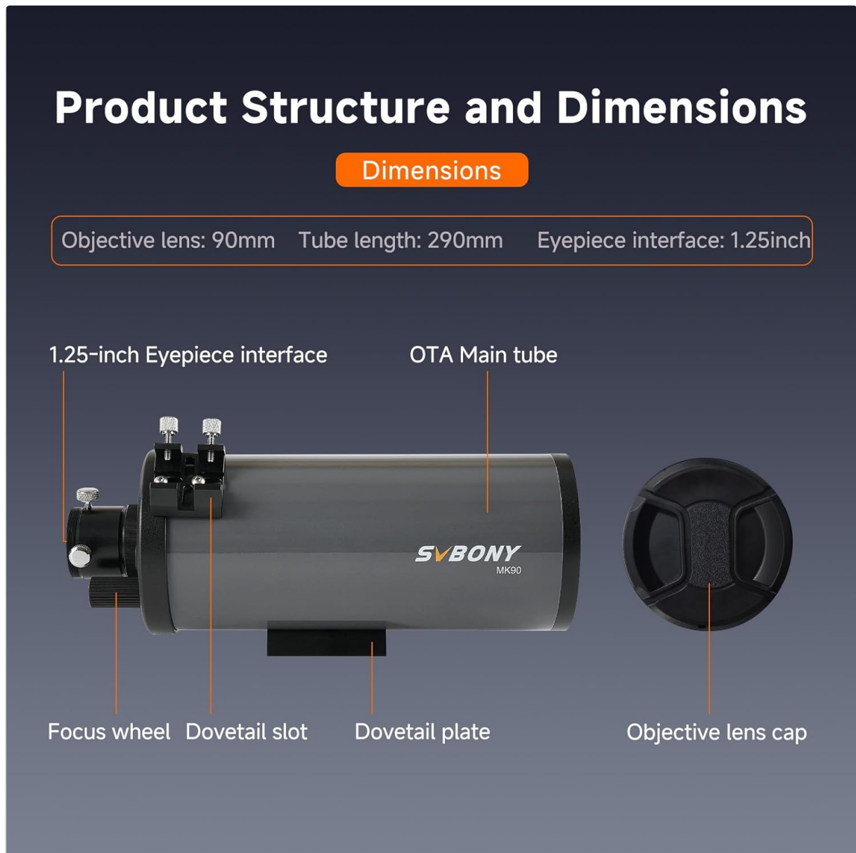
Figure 3: Key structural components and dimensions of the MK90 telescope.
