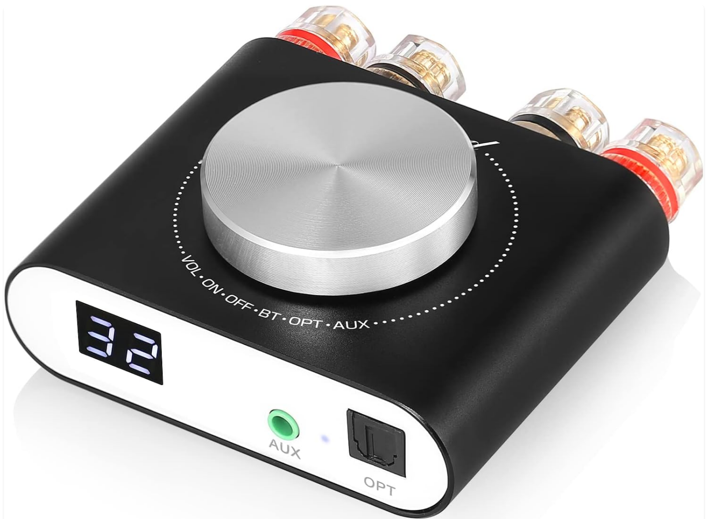
Image: Front view of the Nobsound Q10 amplifier, showcasing its compact design, large volume knob, digital display, AUX input, and Optical input.
