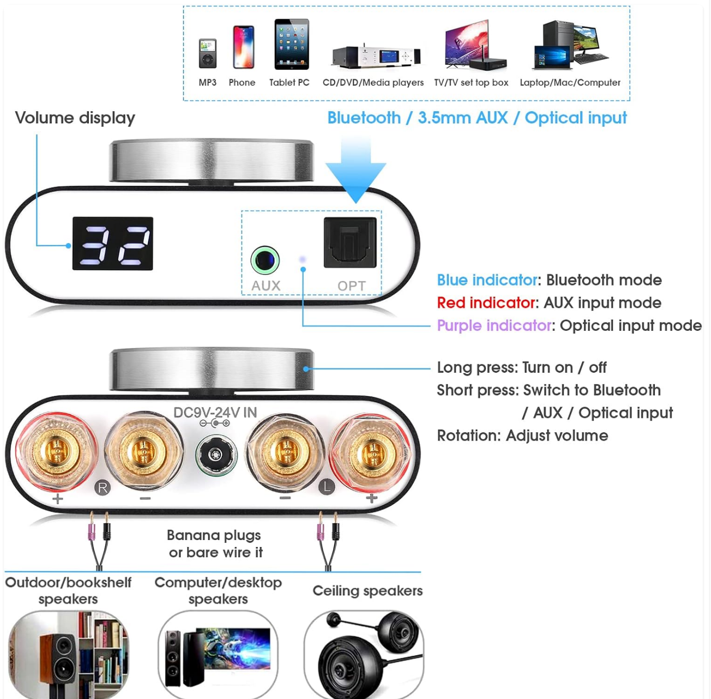
Image: Detailed diagram of the Nobsound Q10's front and back panels, illustrating input/output ports and controls, including speaker connections.
