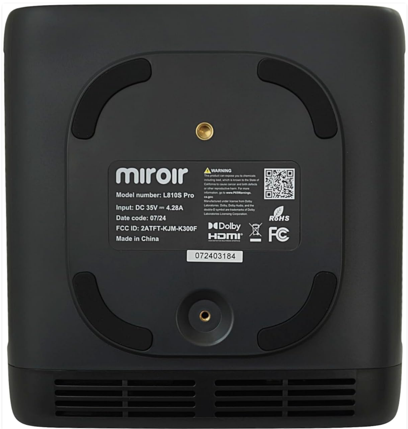
Figure 3: Bottom view of the Miroir L810S Pro Projector, displaying the model number (L810S Pro), input specifications (DC 35V = 4.28A), and various certifications including Dolby Audio and HDMI. A QR code is also visible, linking to Miroir support resources .
