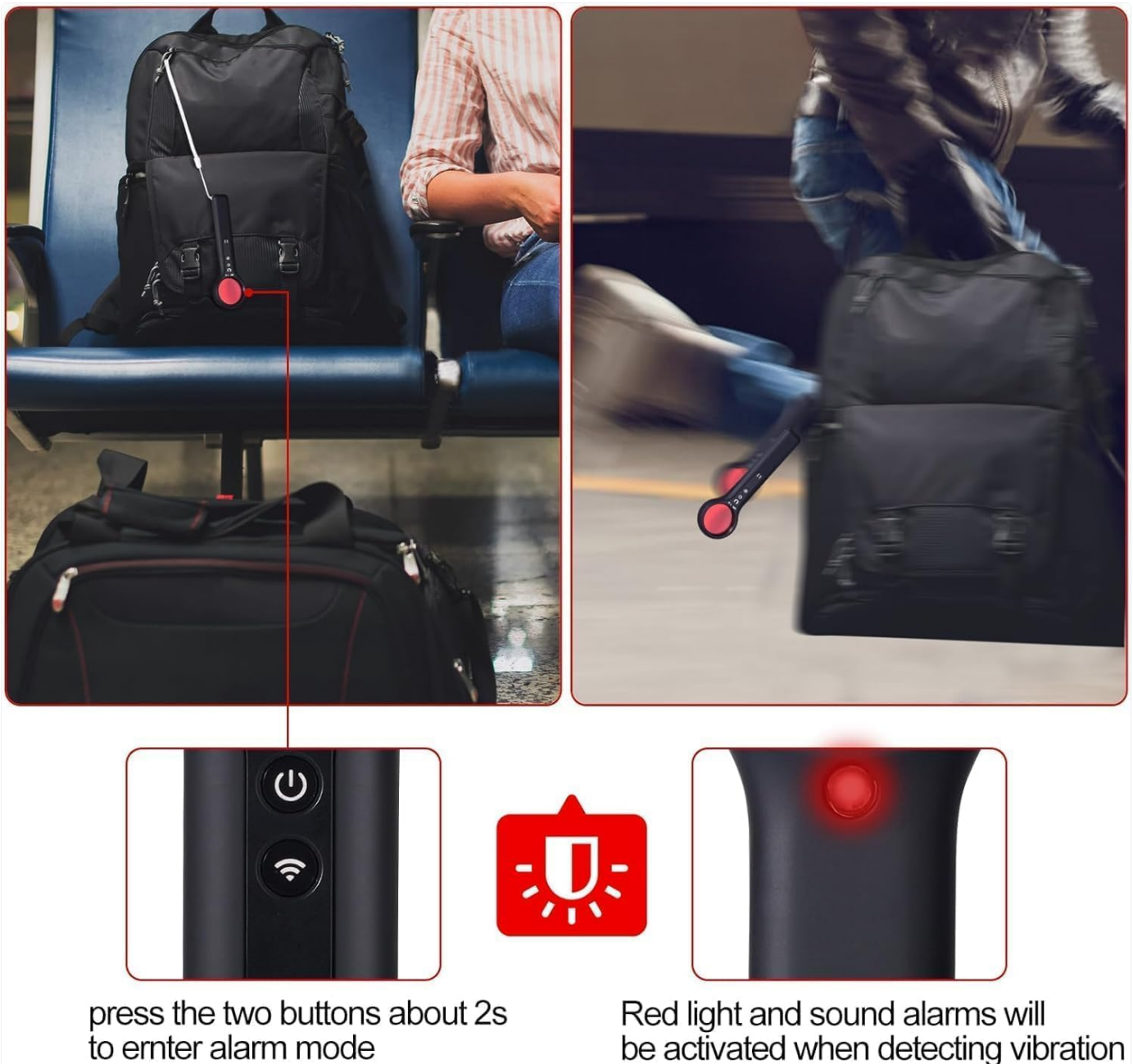
Image 5.4: Anti-Theft Mode. This image illustrates how to activate the anti-theft mode by pressing two buttons for 2 seconds, and shows the device attached to luggage, ready to trigger a red light and sound alarm upon vibration.
