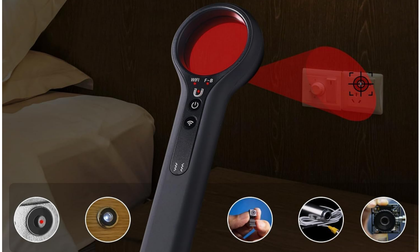
Image 5.2: Hidden Camera Detection. This image illustrates how to use the red viewfinder to scan for hidden camera lenses, which appear as bright red spots.
