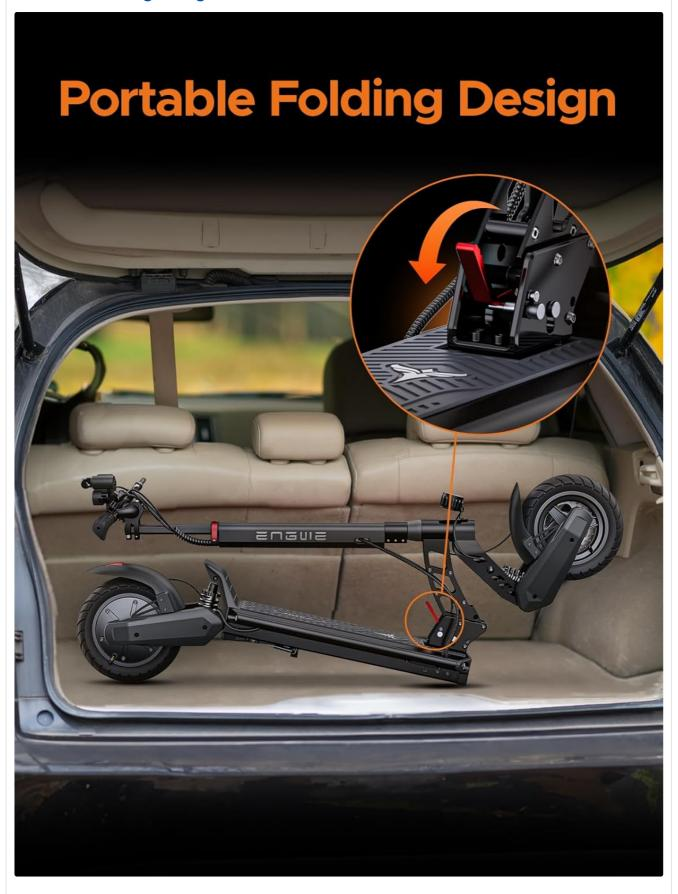
Designed for convenience, the ENGWE Y400 features a foldable mechanism, allowing it to be easily stored in a car trunk or carried up stairs. Its folded dimensions are 52L x 24W x 20H inches, and it weighs 52 lbs, supporting a maximum load of 265 lbs.
