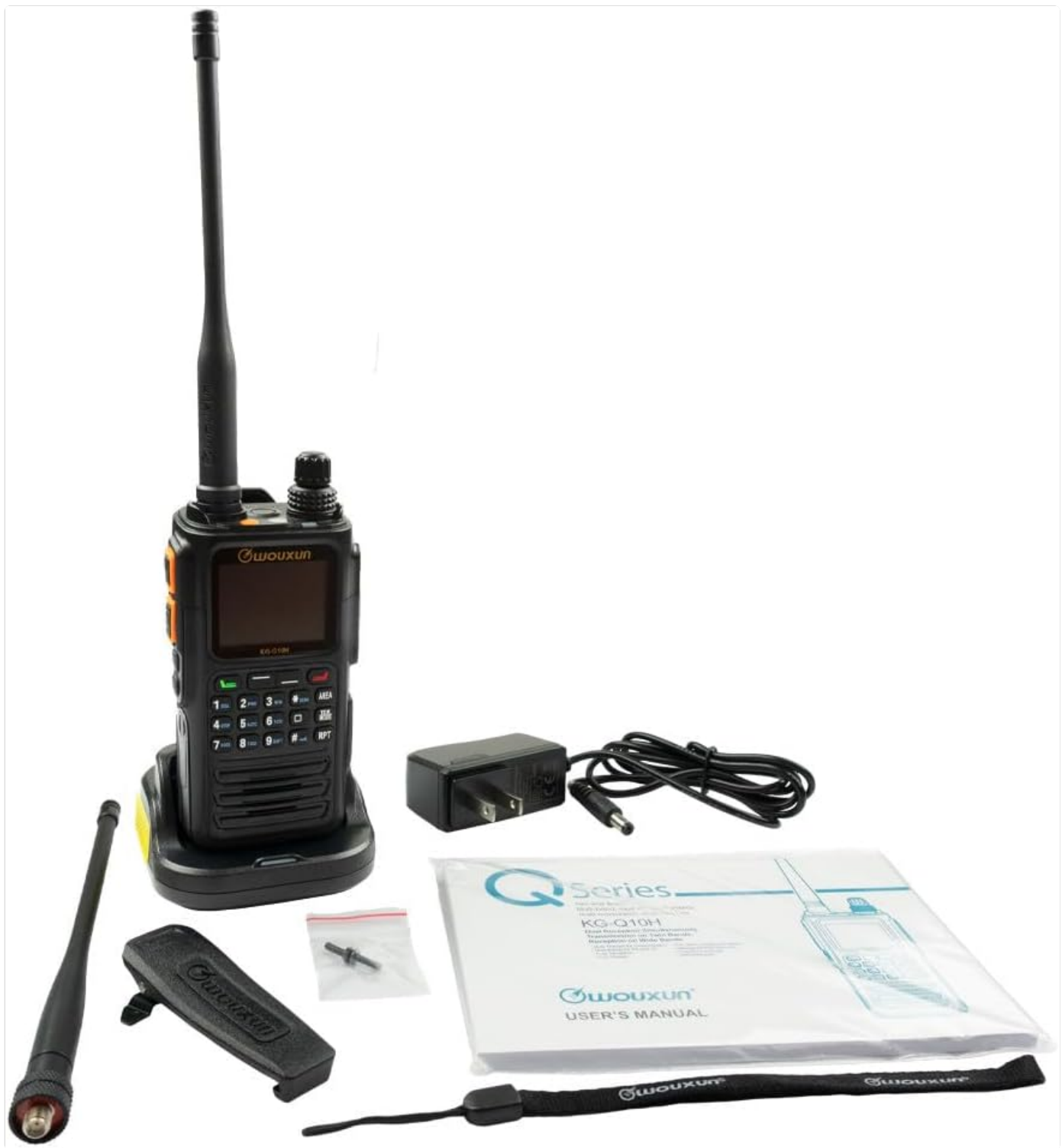
Figure 3.1: Wouxun KG-Q10H radio with its complete set of accessories, including two antennas, battery, charging dock, belt clip, wrist strap, and user manual.
