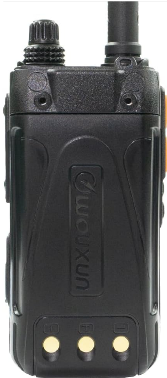
Figure 4.3: Back view of the Wouxun KG-Q10H, showing the battery compartment and belt clip attachment points.
