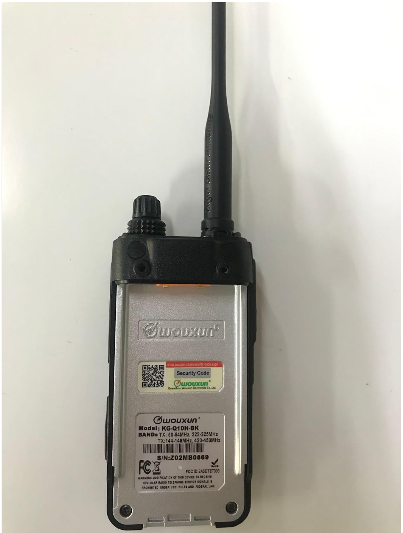
Figure 8.1: Back of the KG-Q10H, displaying the FCC ID and a QR code for security verification on the Wouxun website.
