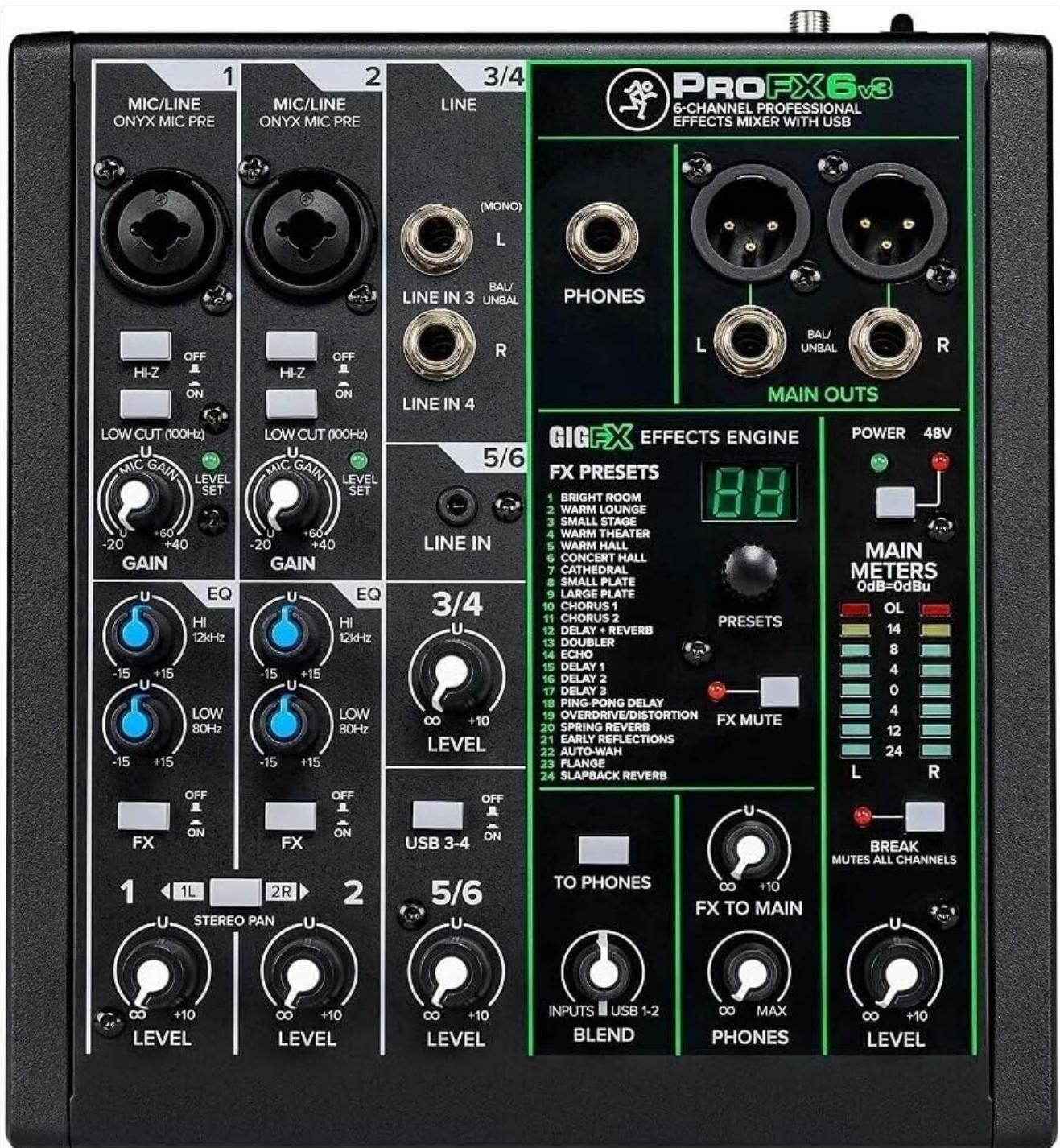
Image: Top-down view of the Mackie ProFX6v3 mixer, highlighting the various controls and ports.
