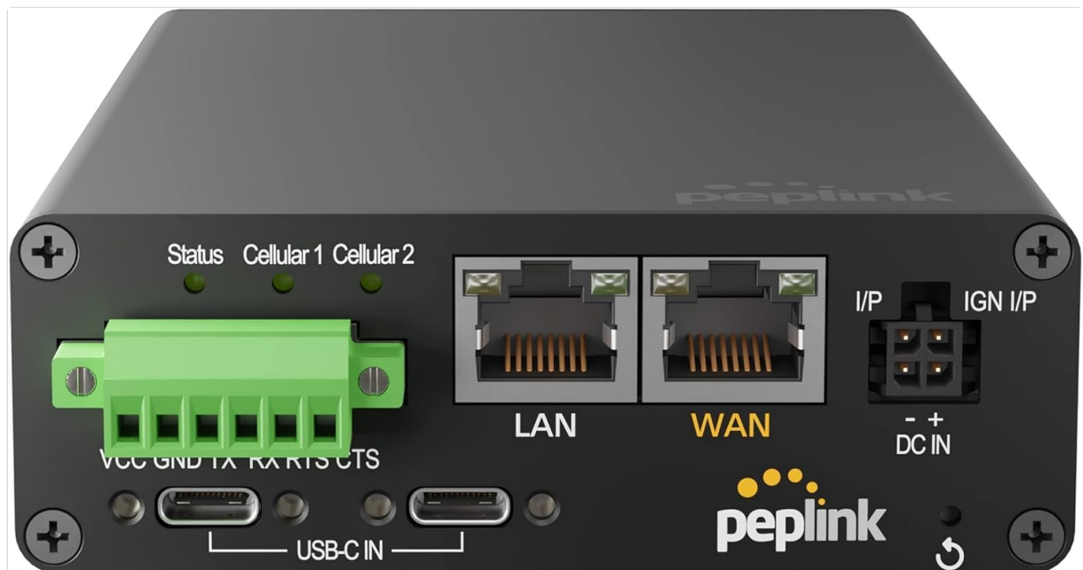
Figure 3.1: Front panel of the MAX Transit Duo Pro, showing LAN, WAN, USB-C, and DC In ports.
