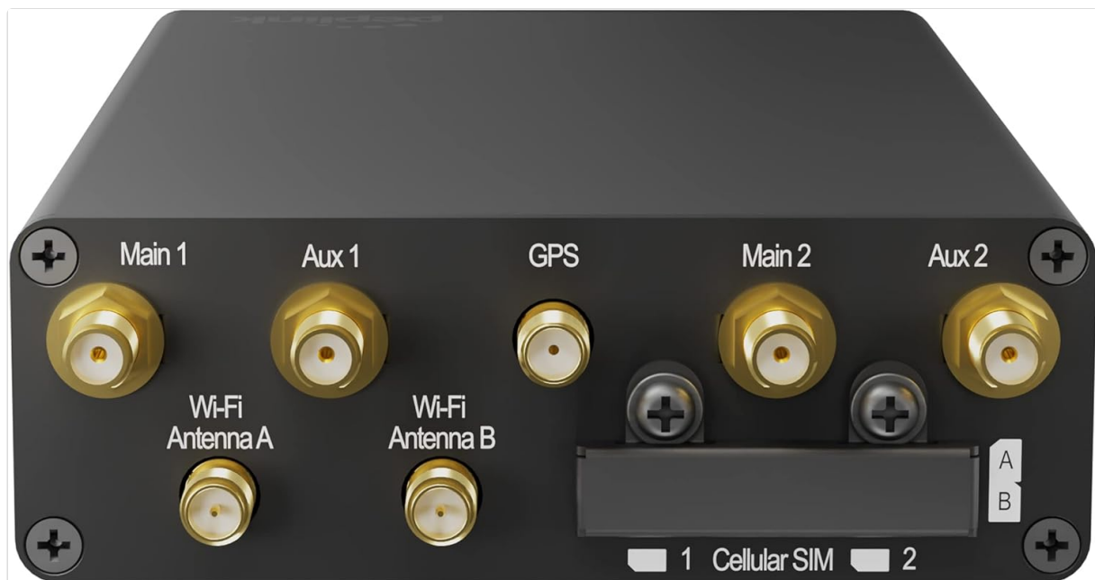
Figure 3.2: Top panel of the MAX Transit Duo Pro, illustrating antenna connectors and dual cellular SIM slots.
