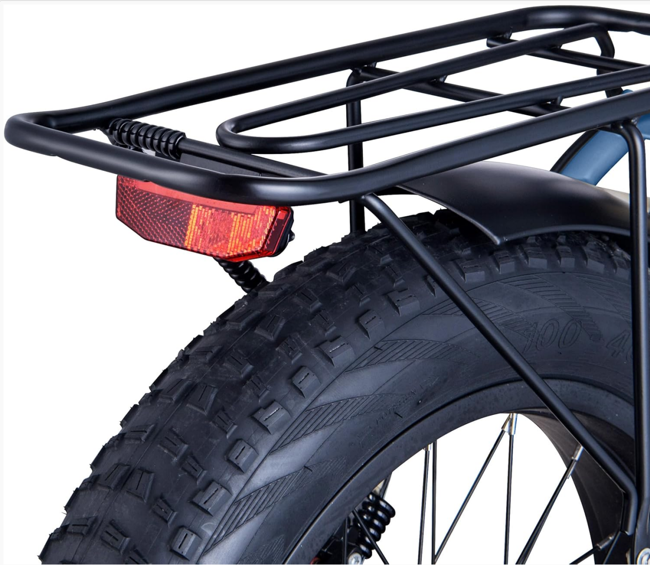
Figure 5.3: Rear rack, taillight, and fat tire. Detail of the rear section of the bike, featuring the sturdy rear rack for carrying items, the integrated taillight for visibility, and the wide fat tire designed for stability on various surfaces.
