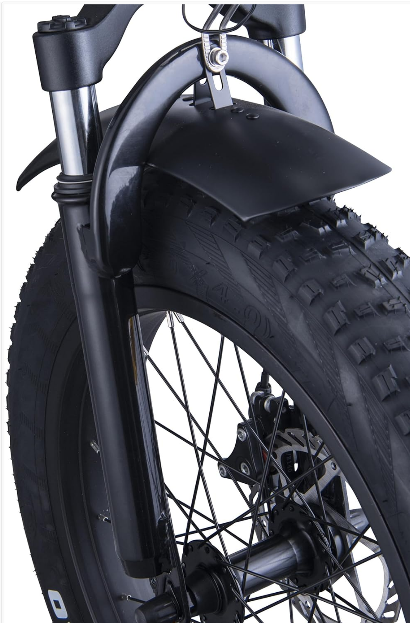
Figure 5.2: Front wheel, suspension fork, and disc brake. A close-up view of the front wheel, showcasing the wide fat tire, the front suspension fork for improved ride comfort, and the disc brake system for effective stopping power.
