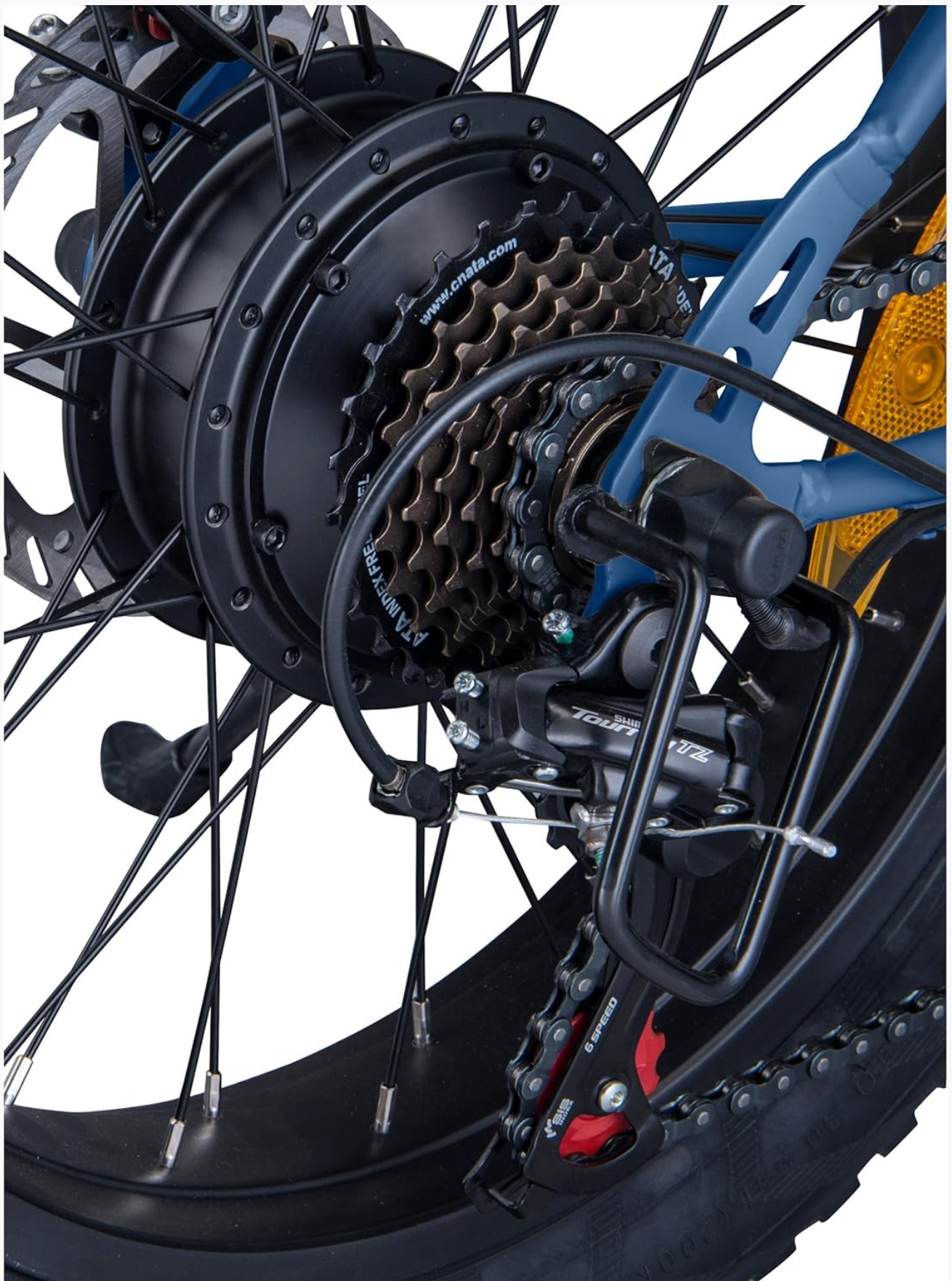
Figure 5.5: Rear wheel, motor, Shimano derailleur, and disc brake. A detailed view of the rear wheel assembly, showing the electric motor, the SHIMANO 6-speed derailleur system for gear changes, and the rear disc brake caliper.
