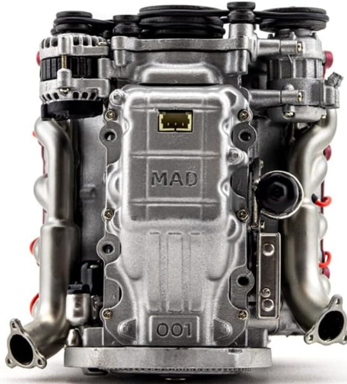
Image 4.1: Rear view of the engine model, highlighting the oil pan structure and power supply interface.
