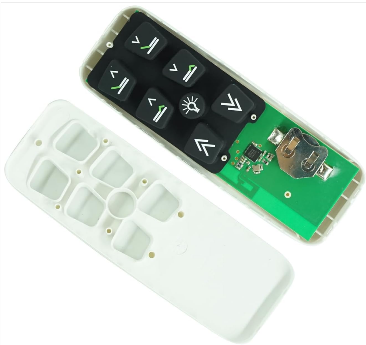
Figure 3: Internal view of the remote control, illustrating the location for battery insertion.
