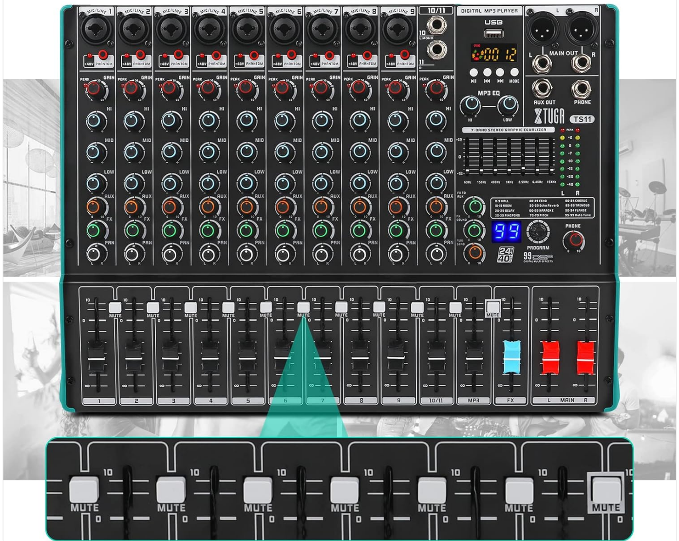
Image: Close-up of the XTUGA TS11 mixer's channel faders and mute buttons, emphasizing the independent mute switch for each channel.
