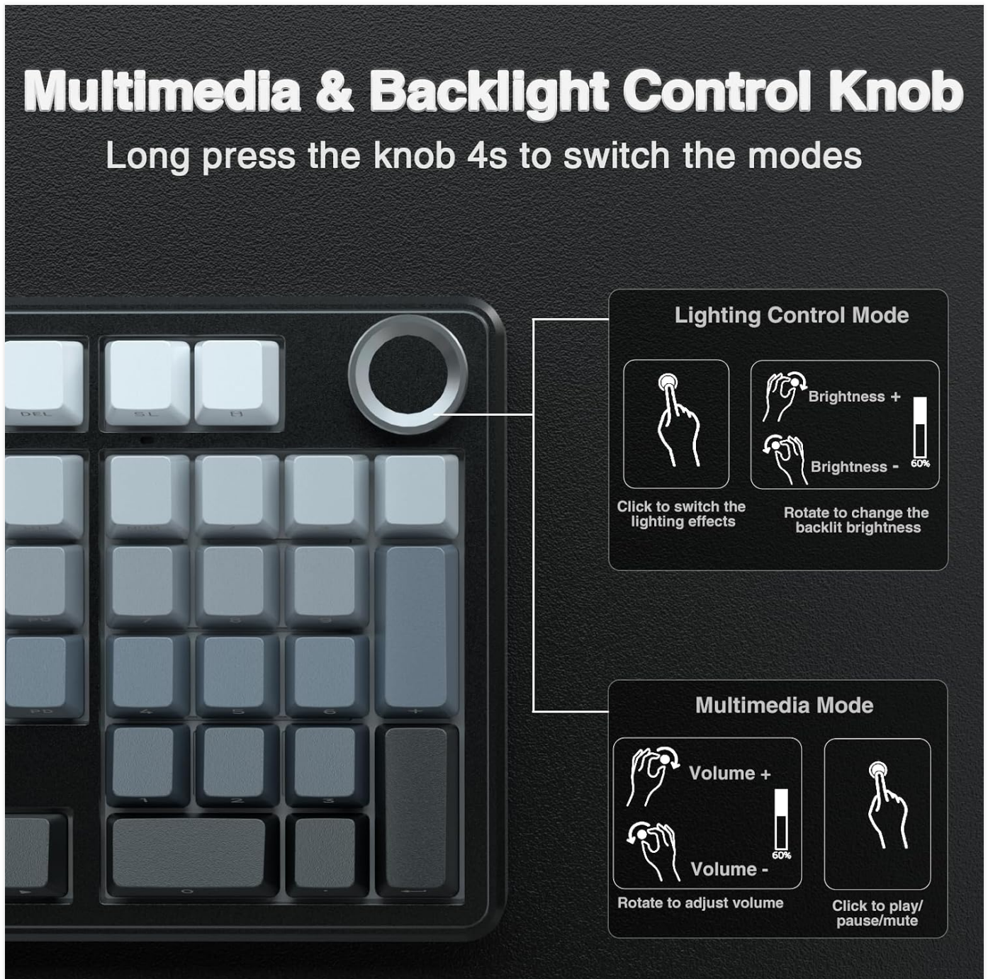
Image: Detailed diagram showing the functions of the multi-function control knob in both Lighting Control Mode (brightness adjustment, lighting effects) and Multimedia Mode (volume control, play/pause).
