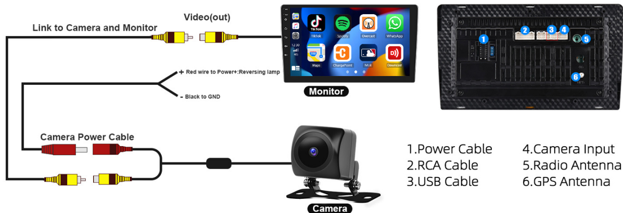
Image: Rear camera wiring diagram for the car stereo.
